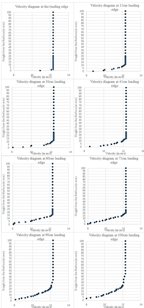
Fig 7: Velocity Profile Plots for 60 Grade at horizontal level
