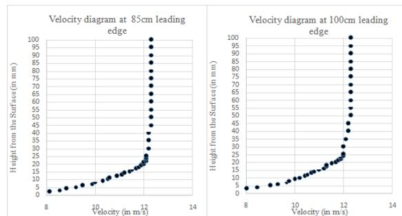
**Fig 4: Velocity Profile Plots for 40 Grade at horizontal level.**
